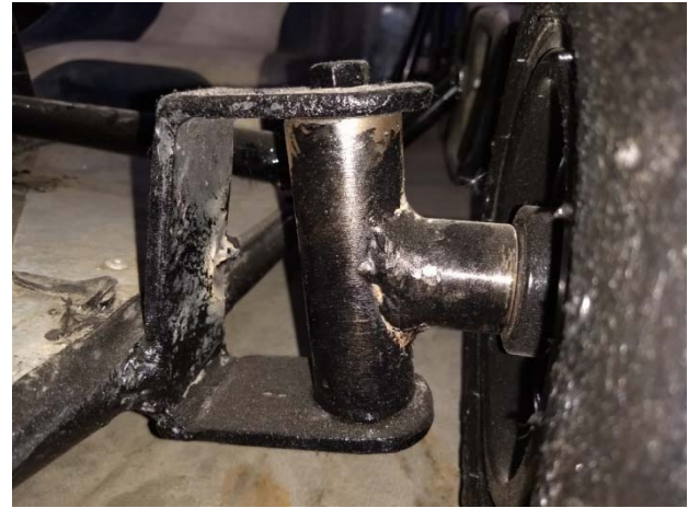
Figure 13: Our Manufactured Stub Axle and Bracket in Go-Kart Vehicle.
